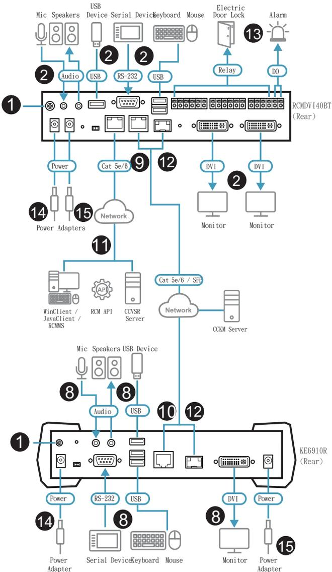
**Note:** The diagram above shows the RCMDVI40BT setup with a KE6910R. The RCMDVI00AT-KE6900AR installation is the same except with one less DVI monitor.
