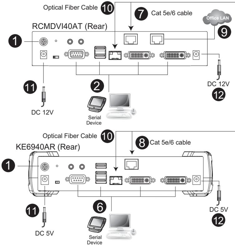
**Note:** The diagram above shows the RCMDVI40AT setup with a KE6940AR. The RCMDVI00AT-KE6900AR installation is the same except with one less DVI monitor.
