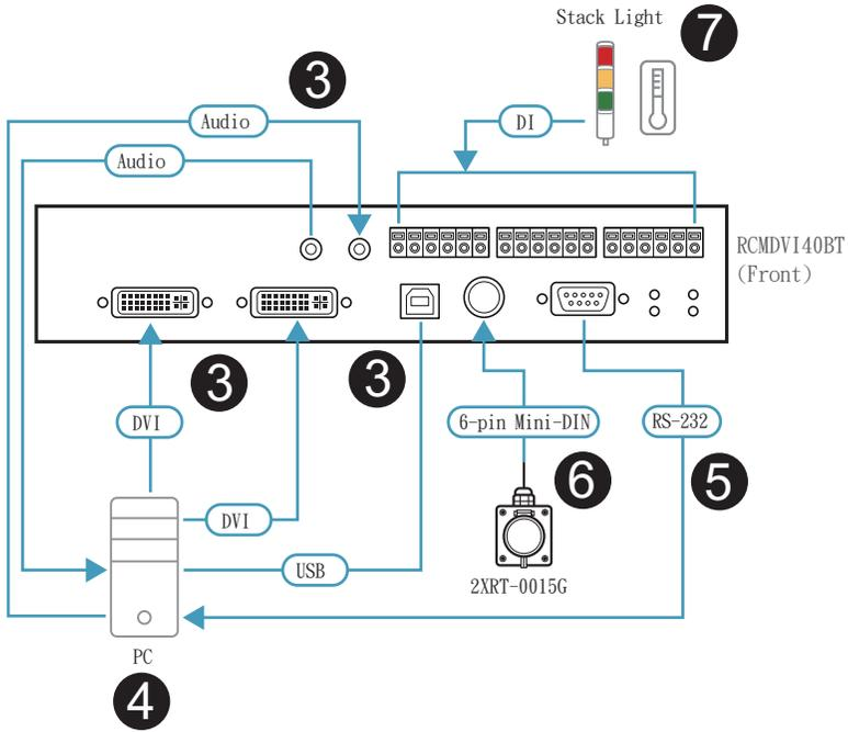
**Note:** The serial port on the transmitter (shown above) connects to the computer; the serial port on the receiver (not shown) connects to a serial device (optional).
